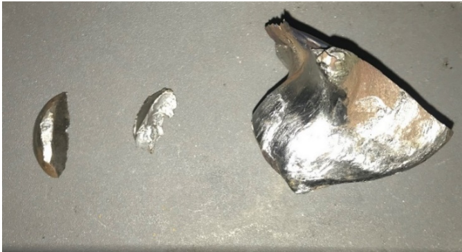
Figure 3. Three small fragments of the A-end cross key from car IC 21013 (Source: Canadian National Railway Company)
