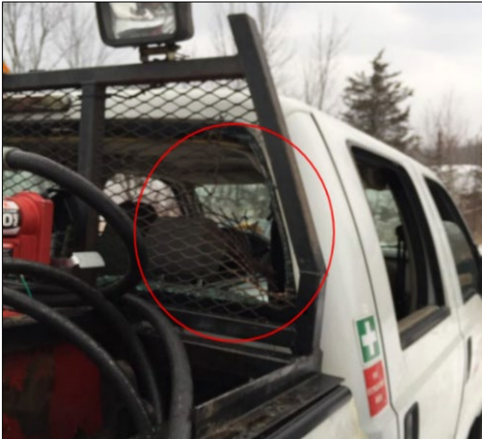
Figure 6. Damage to the protective screening on the rear window of the hi-rail vehicle (Source : CN, with TSB annotations)
