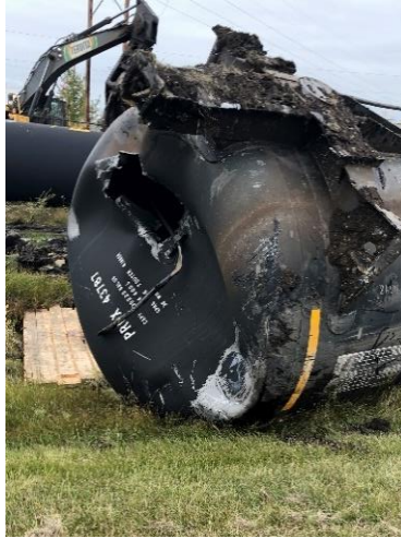
Figure 4. Damage to car PROX 43787 (Source: Canadian Pacific Railway)
