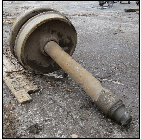
Figure 4. Melted wheelset and wheels of car TR 405202 (Source: TSB)
