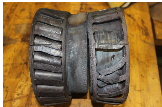
Figure 6. Deformed R1 bearing cage and rollers (Source: TSB)
