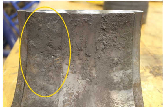
Figure 6. Deformed R1 bearing cage and rollers (Source: TSB)
