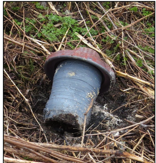
Figure 3. Overheated burnt-off axle journal stub (Source: TSB)
