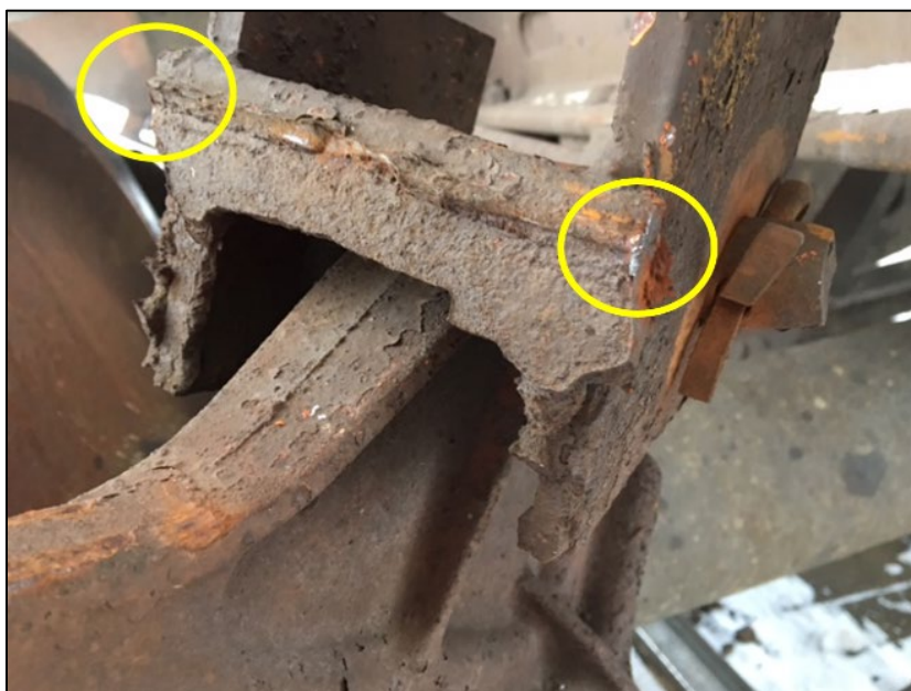
Figure 7. Bell-crank bracket fracture surface containing 2 small zones of fresh fracture (circled) (Source: Canadian National Railway Company, with TSB annotations)
