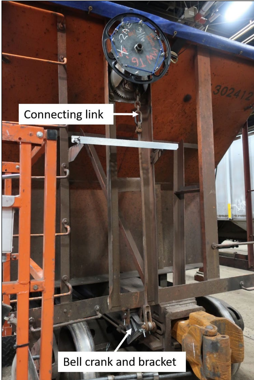
Figure 10. B end of CN 302412 in shop with hand brake applied (Source: TSB)
