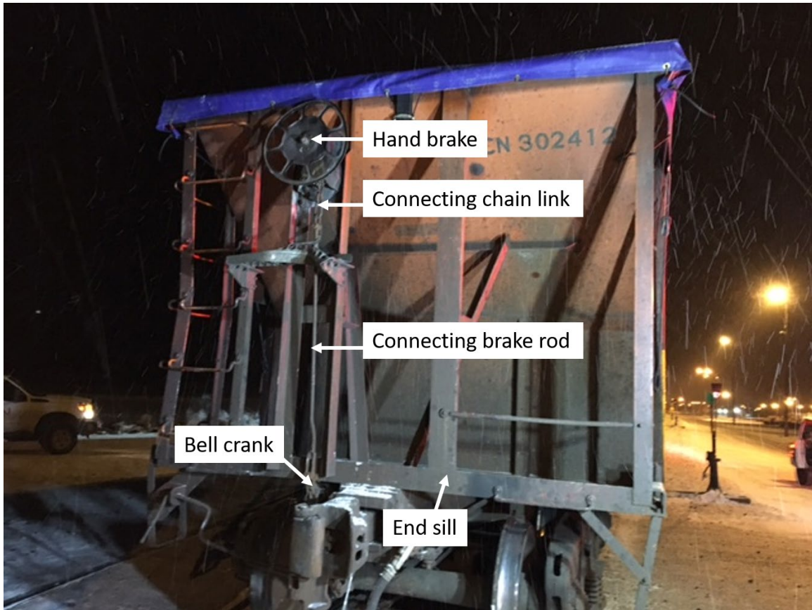
Figure 5. B end of CN 302412, as found about 30 minutes after the accident (Source: Canadian National Railway Company, with TSB annotations)
