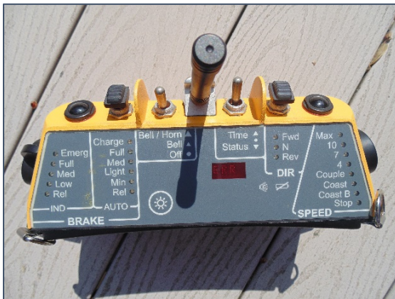
Figure 15. Operator control unit (Source: TSB)_
