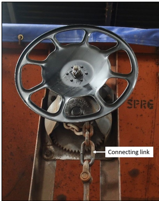
Figure 12. Position of connecting link with hand brake applied and bell-crank bracket cut (Source: TSB)
