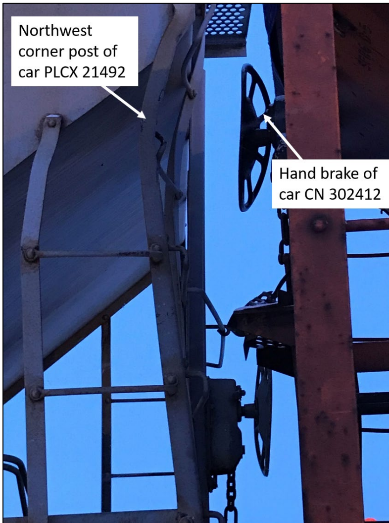
Figure 4. Estimate of how PLCX 21492 and CN 302412 came to rest, as staged the following day (Source: Canadian National Railway Company, with TSB annotations)
