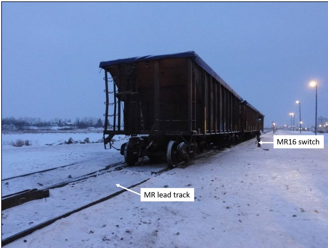
Figure 3. Occurrence open-top hopper cars staged on the MR lead track near the MR16 switch (Source: Canadian National Railway Company, with TSB annotations)
