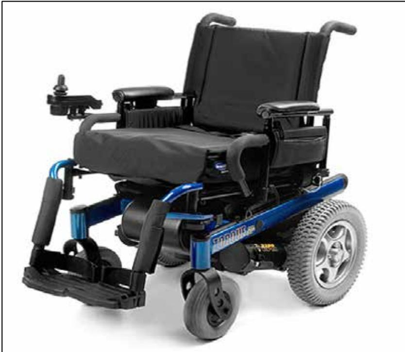
In this occurrence, the motorized wheelchair had 6 wheels: 2 large drive shaft wheels (14 × 3 inches), 2 front caster wheels (8 × 2¼ inches), and 2 rear stability wheels, called anti-tippers (3 × 1¼ inches). The anti-tippers were set approximately 16 inches apart (Figure 12). The weight of the wheelchair, including the battery, was about 275 pounds. The total weight of the occupied wheelchair (i.e., with the pedestrian and all the peripherals) was about 500 pounds.
