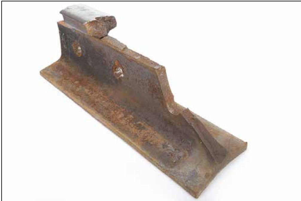
Figure 7. Field-side view of parent rail in the east joint with mating 4-inch-long rail-head fragment
