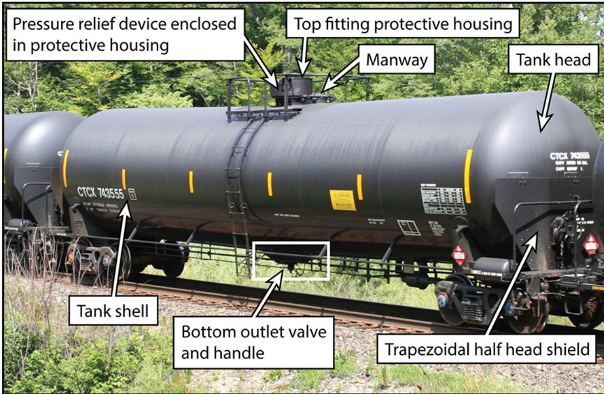
Figure 21. General service Class 111 CPC-1232 tank car arrangement. On all tank cars involved in this occurrence, the pressure relief device for all tank cars involved in this occurrence was located inside of the top fitting protective housing
