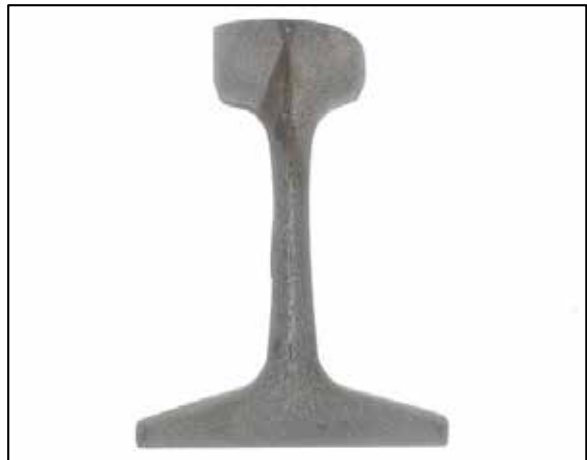
Figure A2. Macro-etched cross-section of the north rail with web streaking and vertical split head defect
