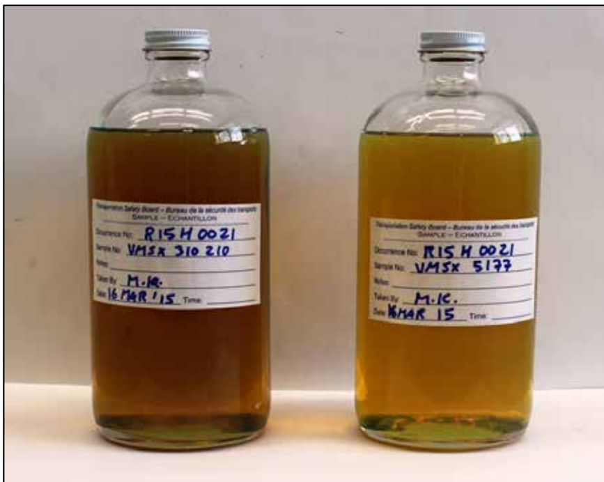
Figure 20. Oil samples from tank cars VMSX 310210 and VMSX 5177
