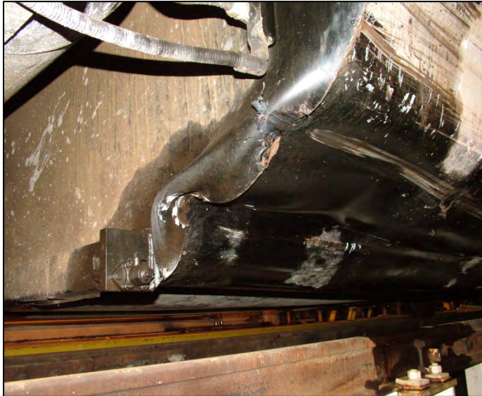
Photo 5. Dented fuel tank on VIA 6444 (source: TSB)
