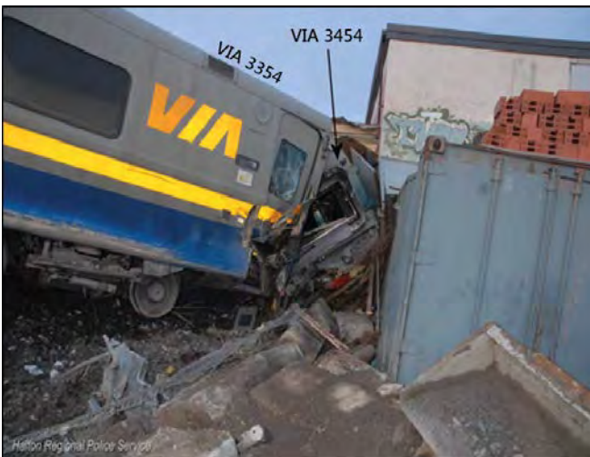
Photo 4. The trailing end door of the 1st coach was cut open while both side doors of the 2nd coach (VIA 3354) were jammed (source: Halton Regional Police)
