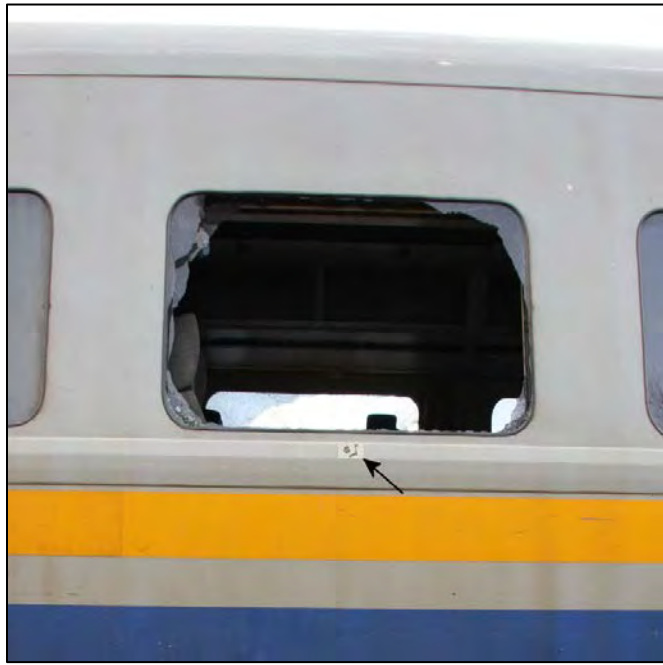
Photo 11. Exterior marking on an emergency window exit (source: TSB)
