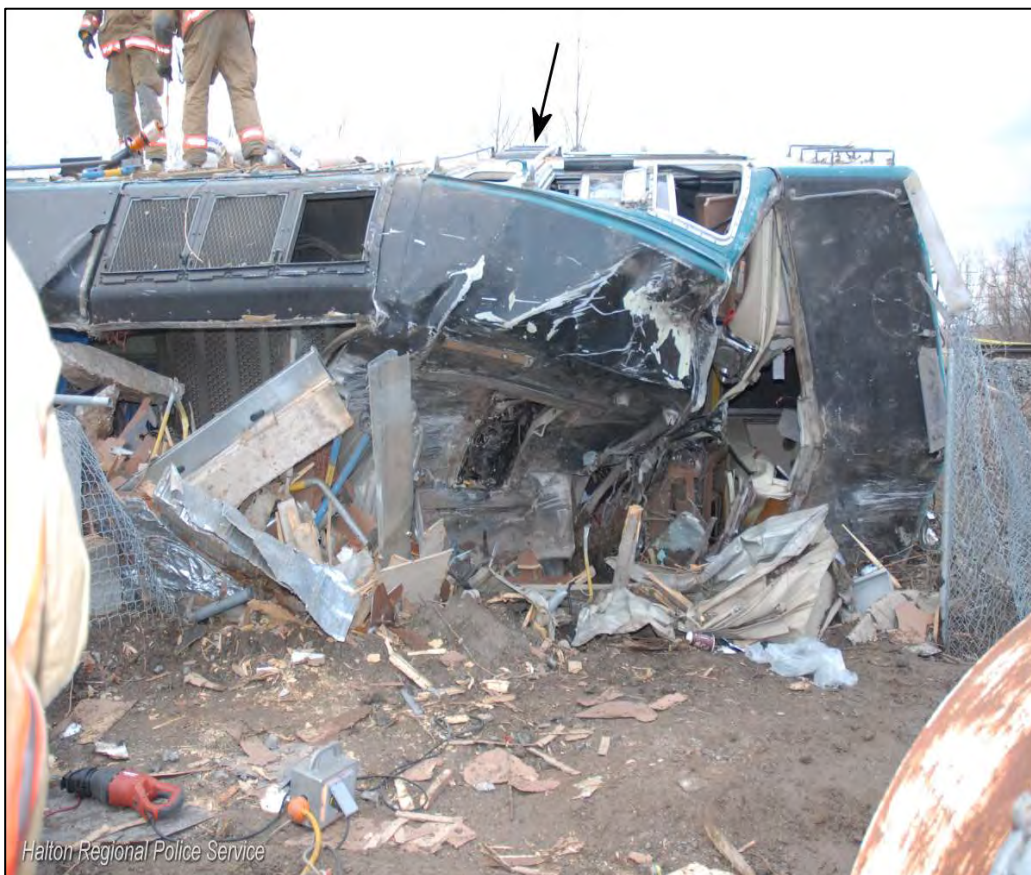
Photo 1. VIA 6444 on its side with collapsed cab roof. ICLE door on top (source: Halton Regional Police).
