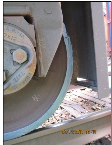
Photo 1b. Close-up of the L3 wheel on DTTX 724638 showing bluing and abrasion on the rim face
