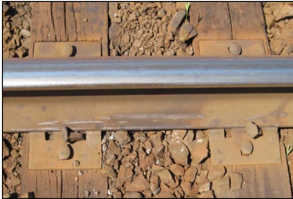
Photo 3a. Bent and lifted gauge-side low rail spikes at the point of derailment
