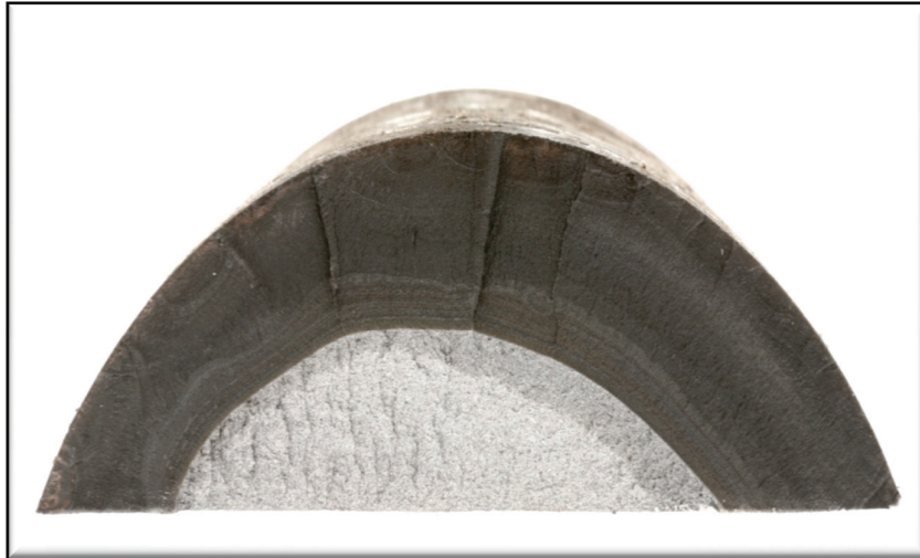
Photo 4. Close-up of secondary crack in axle No. 3
