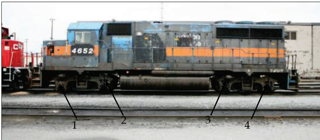
Photo 3. Left side view of CP 4652 showing traction motor assembly position numbering
