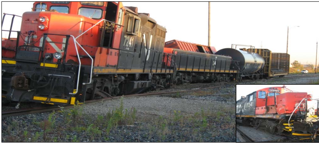
Photo 1. The 2200 West post-derailment. Inset: Damage to CN7241 at point of collision.
