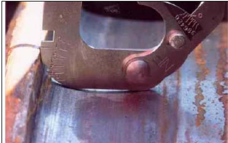
Photo 2. R1 wheel with vertical flange gauge applied
