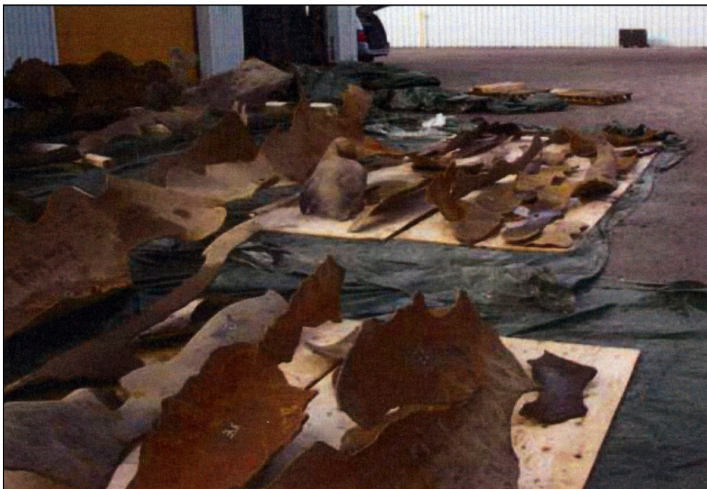
Photo 4. Line 100-1, pipe pieces from the Marten River pipeline failure.
