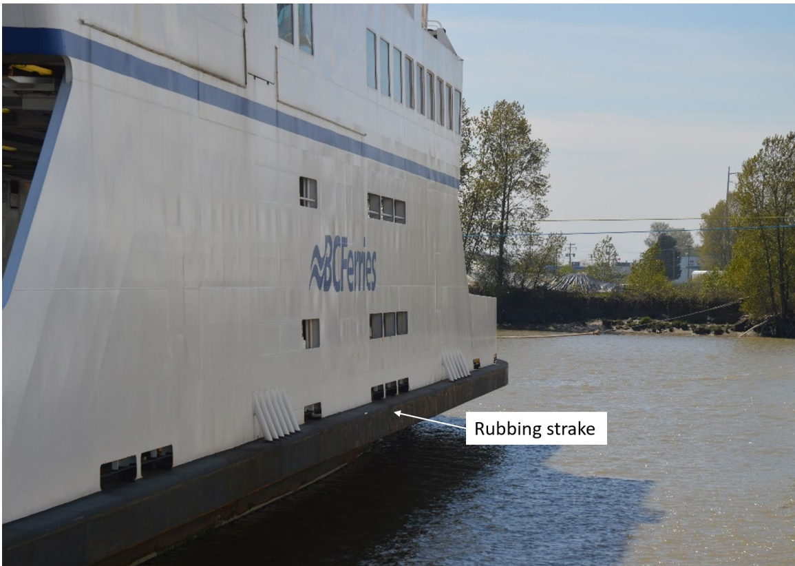
Figure 15. Rubbing strake on the Queen of Cumberland (Source: TSB)
