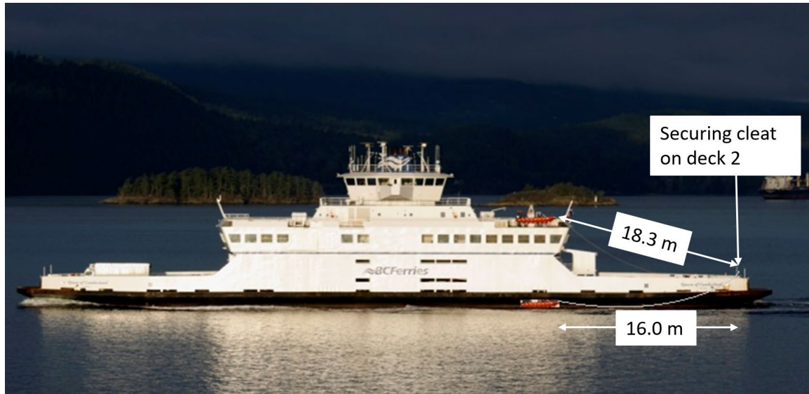
Figure 13. Distance between the rescue boat and the cleat on deck 2 when the rescue boat is in the stowed position versus when it is in the water (Source: Dennis J. Dubinsky, with TSB annotations)
