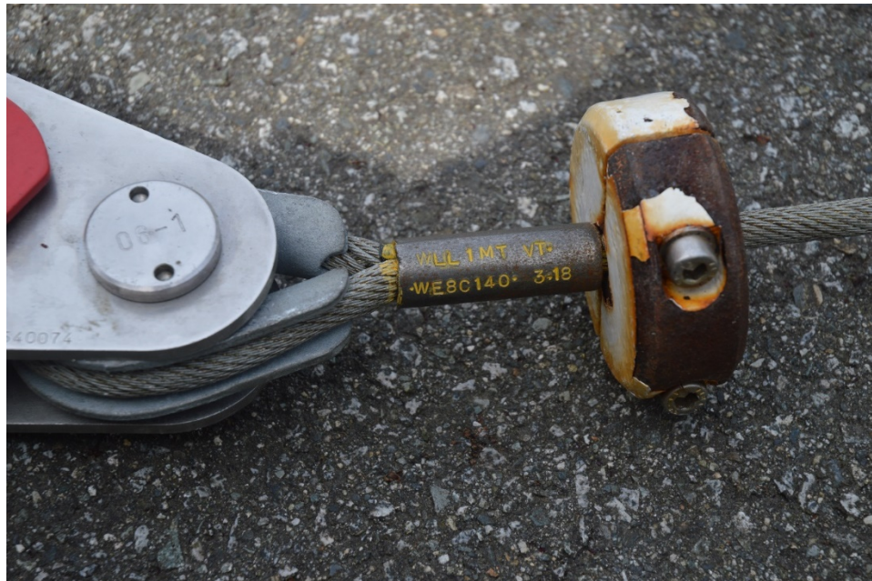
Figure 17. Mechanical splice with safe working load of 1 metric tonne (Source: TSB)
