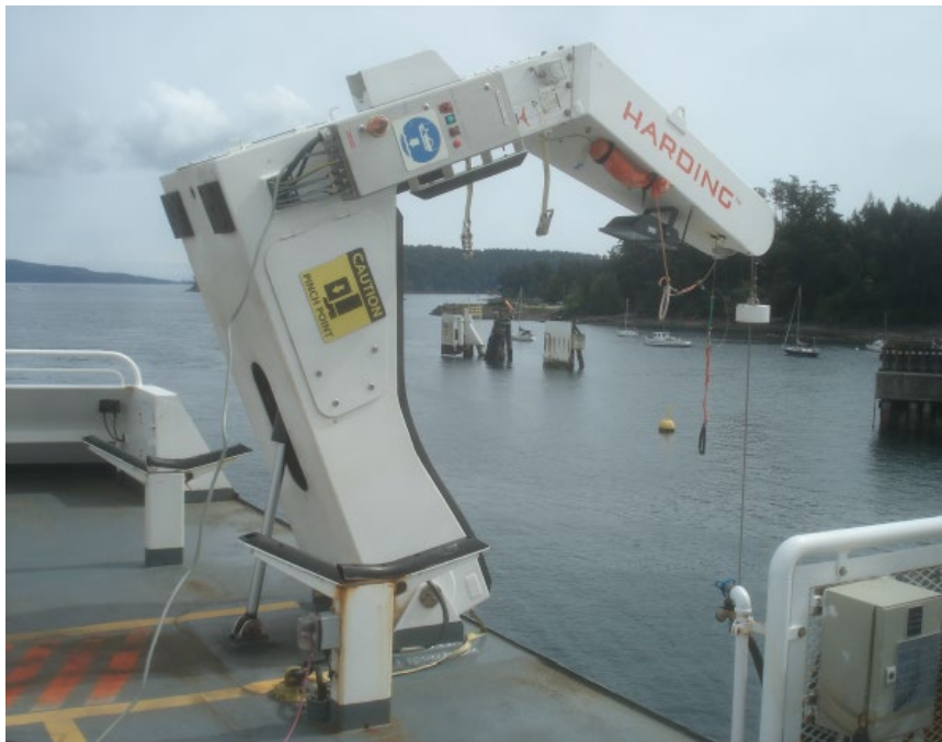
Figure 3. Pivoting davit (Source: TSB)
