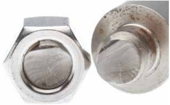
Figure 3. Failed stud showing both halves of the fracture surface
