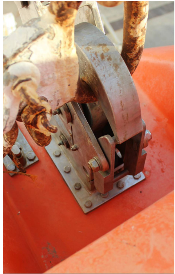
Figure 4. The Northern Ranger's starboard lifeboat release hook fitted with end link (Source: TSB)
