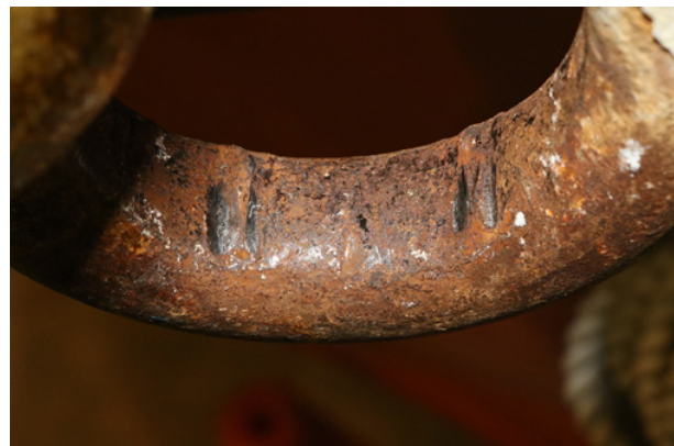
Figure 15. Deformation in the Northern Ranger’s forward end link (Source: TSB)
