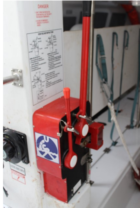
Figure 5. On- or off-load release mechanism and instructions in the Northern Ranger's starboard lifeboat (Source: TSB)
