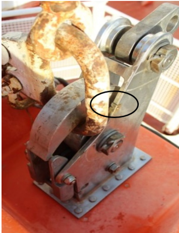
Figure 9. Lifeboat forward release hook in the closed position, with release hook lock-position indicators aligned (black circle). Operator's view would be obscured by end link. (Source: TSB)
