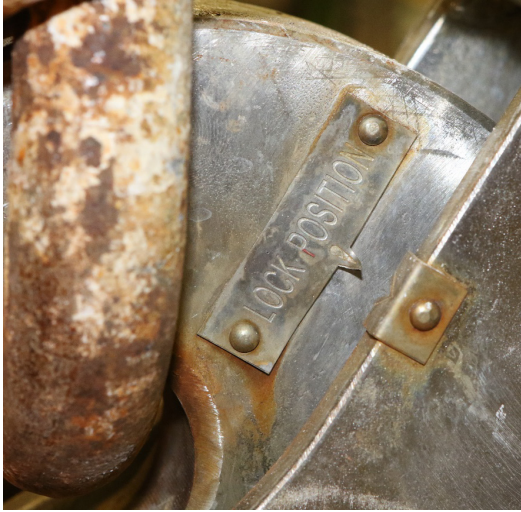
Figure 11. Close-up of forward release hook lock-position indicator (aligned in reset and locked position) (Source: TSB)
