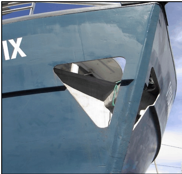
Photo 5. Examples of vessels' overall length being reduced by opening the end compartment to the sea. This can compromise the watertight integrity of those vessels. These modifications are done to meet the DFO length restrictions. Note: Openings made in the bow section of the vessel on the photo to the left. Drain holes at the bottom of the triangular plate on the photo to the right.
