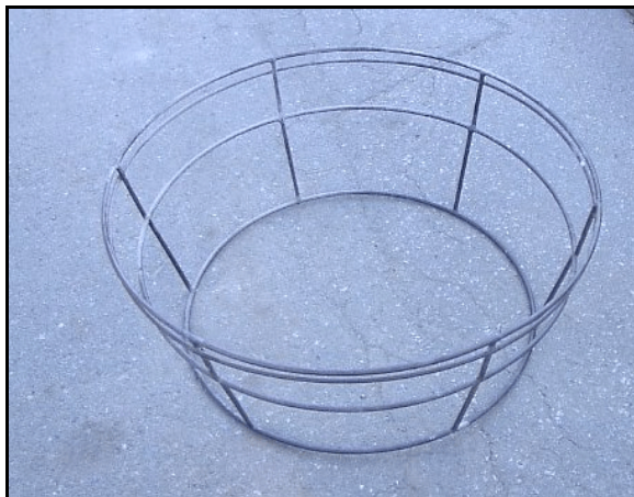
Photo 2. Shell of trap before cordage is added
