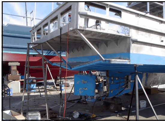
Photo 4. Examples of platform deck extension to accommodate extra traps
