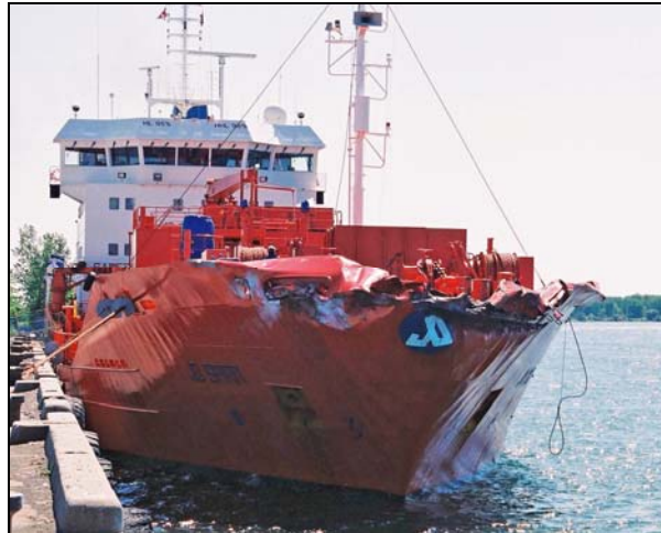
Photo 3. Bow damage on Jo Spirit
