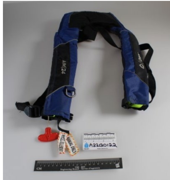
Figure 4. Example of an Onyx A/M-24 manual/automatic personal flotation device recovered from the occurrence aircraft. This is the same model as the one the occurrence pilot had. (Source: TSB)
