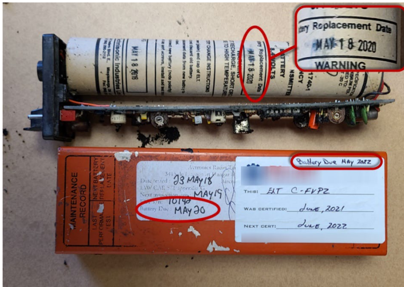
Figure 4. Photo of the emergency locator transmitter showing the replacement date of the internal battery in the close-up (Source: TSB)
