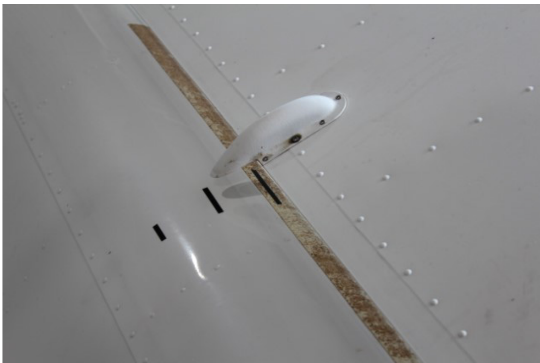
Figure 6. The 10°, 20°, and 30° flap indicator markings on the left wing of an exemplar aircraft. The flap position shown is indicating 30°. (Source: TSB)
