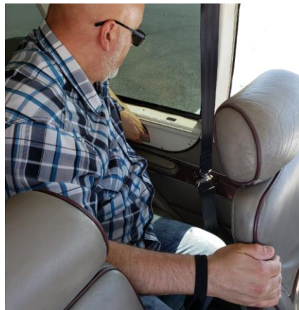
Figure 11. Location of emergency exit window handle during testing (Source: TSB)
