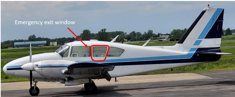
Figure 5. Side view of the Piper PA-23-250 aircraft showing the emergency exit window (Source: TSB)
