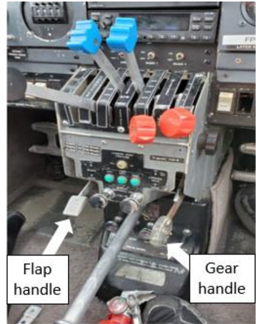
Figure 2. View of landing gear and flap handles (Source: TSB)
