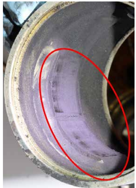
Figure 4. Scarring marks on stator
