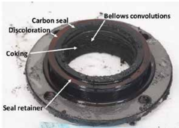
Figure 2. Air-oil seal assembly (stationary seal), showing discoloration and coking
