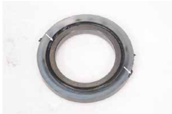
Figure 3. Air-oil seal assembly (rotor seal), with coking indicated by the white arrows
