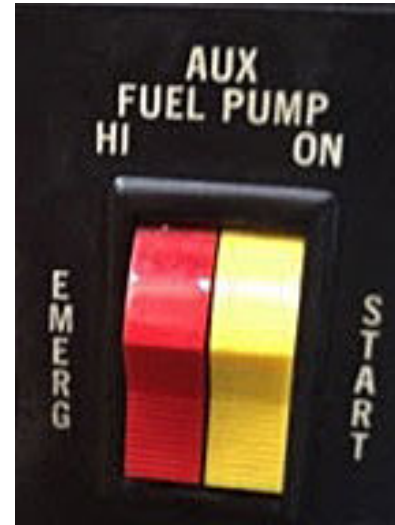
Figure 3. Auxiliary fuel pump switch (Source: Maurice Gunderson)
