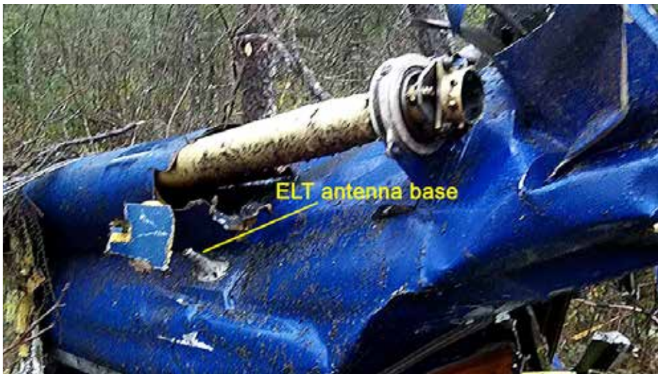
Figure 6. A frame grab from a field video of the wreckage showing the severed emergency locator transmitter (ELT) antenna
