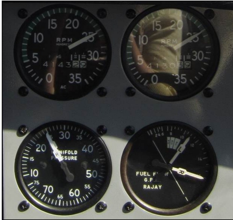
Photo 2. Fuel-flow indicator, 23 March 2012
