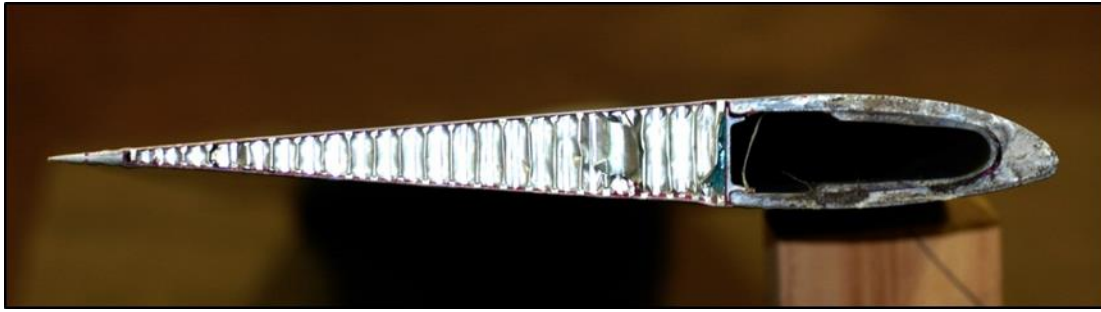
Photo 2. Cross-section of fractured blade (blade station 121)
