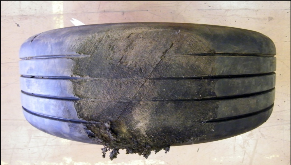
Photo 3. Damage seen on main landing gear tire no. 2 was evident on all 4 main landing gear tires.
