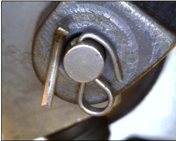
Photo 4. Fractured cotter pin
