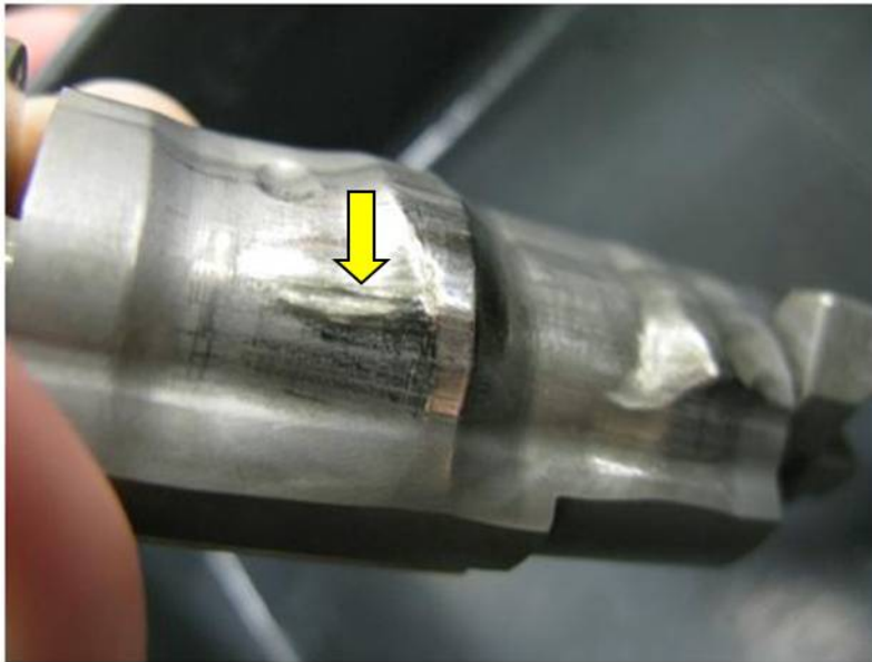
Photo 6. Wear on 3D cam
