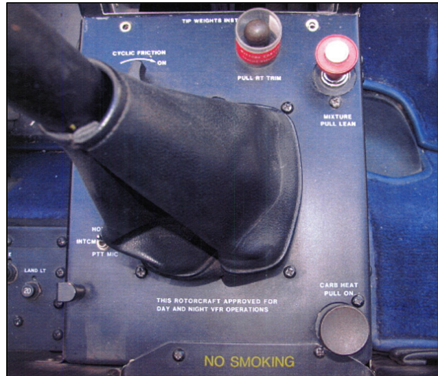
Photo 1. Centre pedestal with mixture control at upper right and carburetor heat control at lower right
