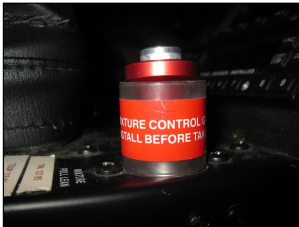
Photo 2. Mixture control pushed in to full rich with guard installed
