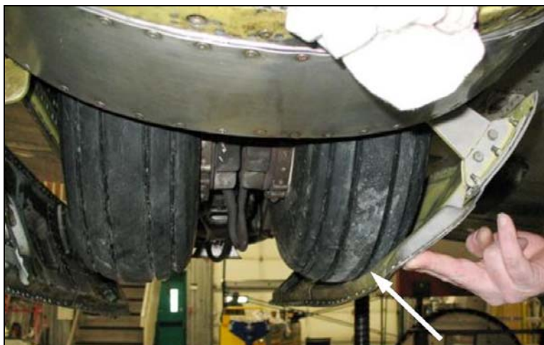
Photo 2. Area of tire-to-gear-door interference
