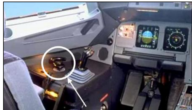
Photo 5. A320 Nose wheel tiller
