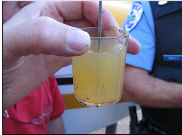
Photo 1. Water from gascolator
