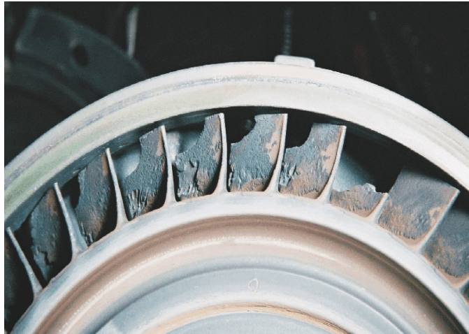
Photo 1. Sulfidation of number 1 GP turbine. Engine compressor washing is recommended in corrosive and dirty environments. It is also prescribed when engine performance has depreciated, as noted from power assurance checks. However, there has been concern that some tap water can in itself be corrosive. Operators rarely do compressor washes when their helicopters are operating away from a salt environment. They will wash compressors when they can see dirt building up at the air intake, or when an engine is performing below specifications. It is not clear if compressor washing effectively cleans the GP turbine wheel.
