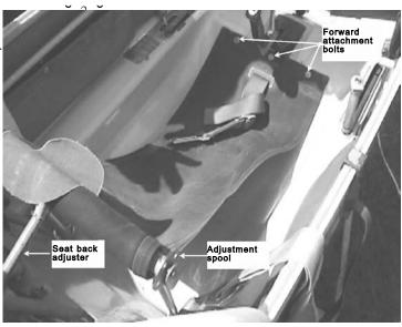
possible to quantify the extent to which this thread damage reduced the clamping strength of the anchor nuts. It could not be determined, through engineering analysis of the seat and attachment hardware, whether the bolts pulled out prior to ground impact or as a result of ground impact loads.
