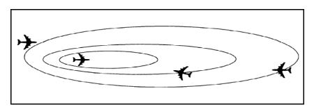
intruding aircraft enters the caution area or the warning area. The dimensions of these two areas vary according to closure speed. When the system predicts that an intruder will enter the collision area within 20 to 48 seconds (the caution area), the TCAS issues a TA to the pilot. A TA provides information on nearby traffic and is designed to help the crew visually detect conflicting traffic and to warn a pilot that an RA may follow.
