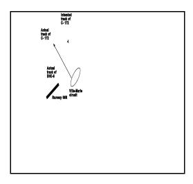
that time, the Cessna, still on the tower frequency, was crossing the departure path of Runway 06R, about 6 nm from the runway end on a northwesterly heading.
