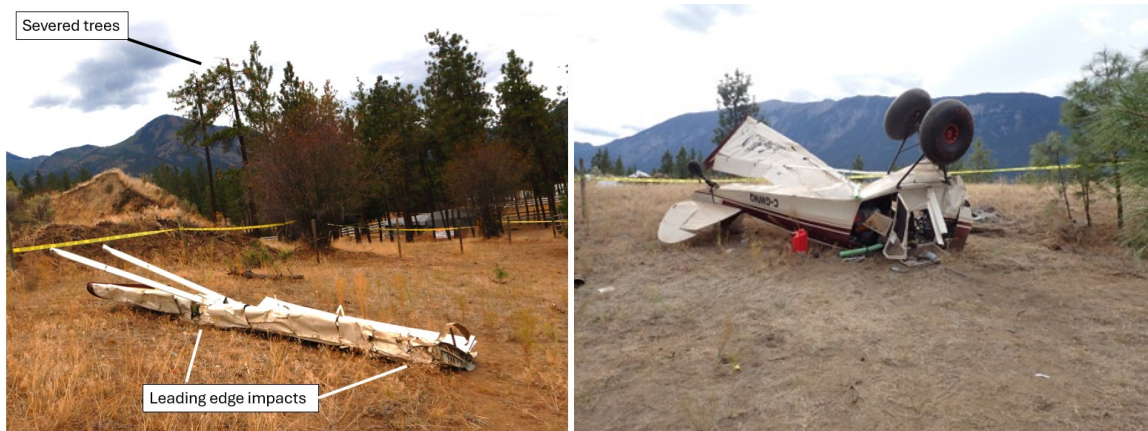
Figure 3. Left wing with leading edge impacts and severed trees (Source: TSB) Figure 4. Wreckage at accident site (Source: TSB)
