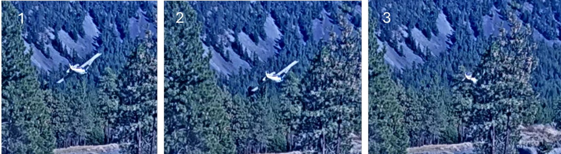
Figure 2. Still images showing the occurrence aircraft's collision with trees (Source: Third party, with permission and with TSB annotations)
