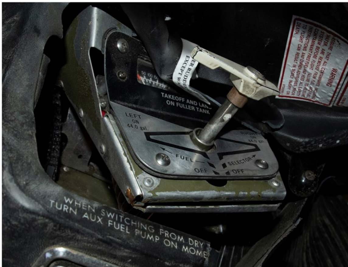
Figure 4. Occurrence aircraft's fuel selector handle in the LEFT ON position, as found post occurrence (Source: TSB)
