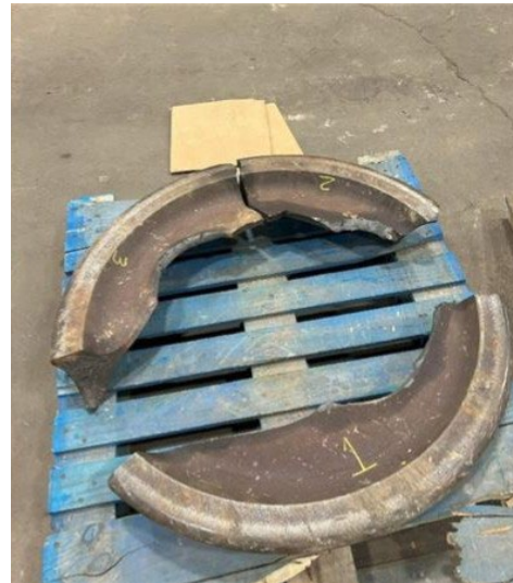
Figure 2. Recovered fragments of the L2 wheel of car NKLX 200817 (Source: TSB)
