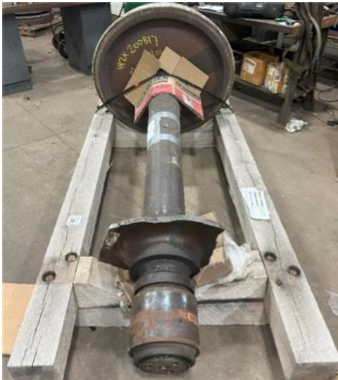
Figure 1. Recovered R2/L2 wheel set of car NKLX 200817 (Source: TSB)
