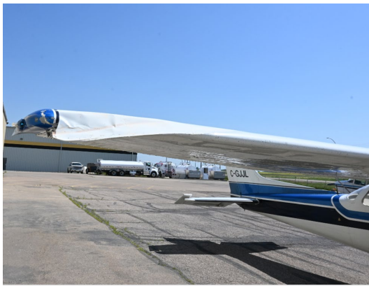
Figure 2. Damage to right wing tip on the Cessna 172 (Source: TSB)
