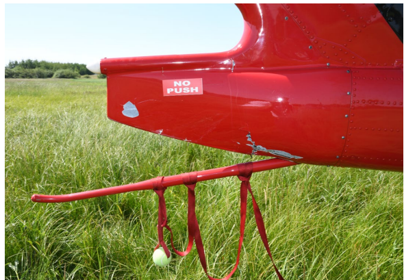
Figure 3. Damage to tail skid area on the Bell 212 (Source: TSB)
