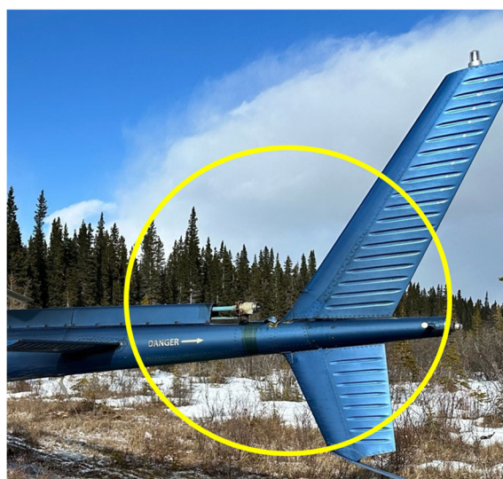
Figure 4. Occurrence helicopter's tail boom, showing the "DANGER" and arrow markings as well as the approximate radius of the tail rotor arc (Source: Heli Explore Inc., with TSB annotations)
