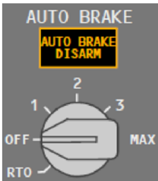
Figure 10. Autobrake selector and indicator (Source: The Boeing Company)
