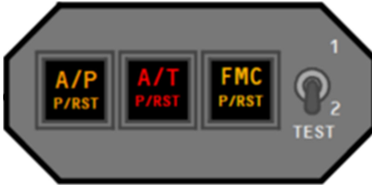
Figure 6. Autopilot (A/P) and autothrottle (A/T) indicator, which houses the A/P and A/T disengage lights (Source: The Boeing Company)
