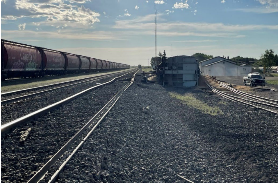
Figure 2. View from the north side of the main track, looking west, showing the second derailed car rolled on its side and, further in the distance, the first derailed car, which remained upright and coupled to the head end of the train (Source: Canadian Pacific)
