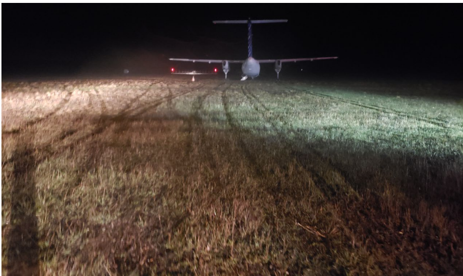
Figure 2. Occurrence aircraft after the runway overrun, photo taken from the end of the paved surface of Runway 12 (Source: Porter Airlines Inc.)
