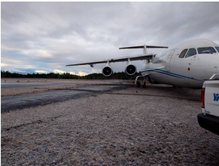
Figure 1. The occurrence aircraft's final position after the overrun, 30 m beyond the end of the runway (Source: Third party, with permission)
