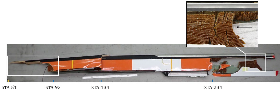
Figure 14. Main rotor blade 0517B highlighting the toothpick shape of the wood spar failure at the blade root and the longitudinal compression of the honeycomb core at the blade tip (Source: TSB)
