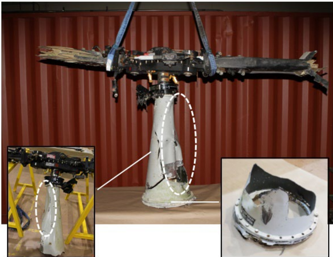
Figure 12. Right-rotor pylon with the hub and blade roots indicating the 2 broken pieces of the pylon and highlighting the compressive buckling on the outboard side (Source: TSB)
