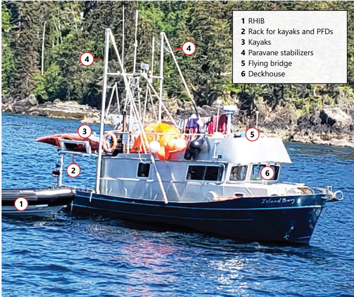
Figure 1. A picture of the Island Bay showing the rigid-hulled inflatable boat, rack for kayaks and personal flotation devices, kayaks, paravane stabilizers, flying bridge, and deckhouse (Source: Royal Canadian Mounted Police, with TSB annotations)
