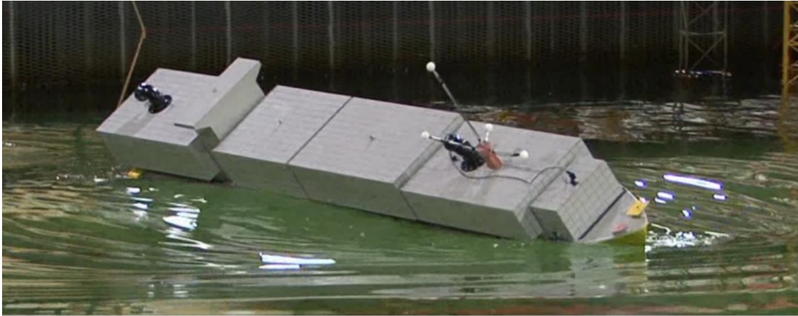
Figure 18. Still photo of the ZIM Kingston model rolling to large angles during tests. Note that the level of water is reaching the containers on the deck; at full scale, this would be considered a green water event (Source: National Research Council Canada)
