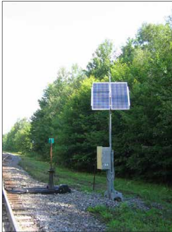
Photo 7. Switch position detection at Salomé
